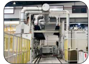
IPSEN Carburising Equipment(Germany-made)
